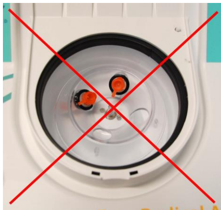
Unbalanced positioning (incorrect)
